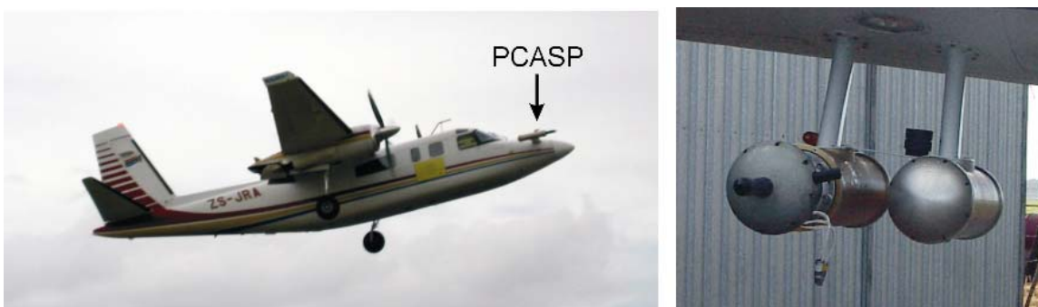
Figure N.3: Left: The Passive Cavity Aerosol Spectrometer Probe (PCASP), mounted on the nose of the Aerocommander during UAE 2 . Right: A close-up of the PCASP (mounted on the wing in this case)
