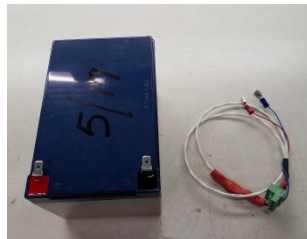
External Battery (12V 12Amp Hr.) and Cable
