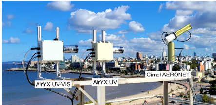
Figure 2. Instruments are installed on the roof of the Faculty of Engineering building located in Montevideo, Uruguay (34.9175° S, 56.1669° W). AirYX equipments are Multi-Axis Differential Optical Absorption Spectroscopy (MAX-DOAS).
