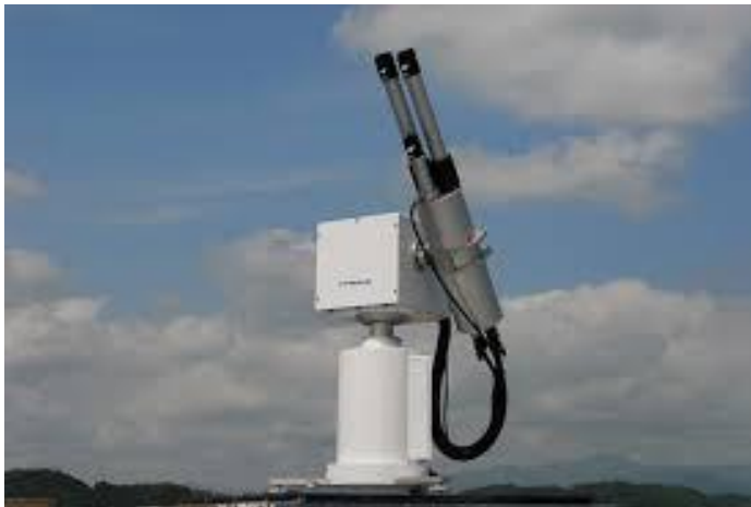
Prede-POM is the standard Skynet sun-sky photometer
