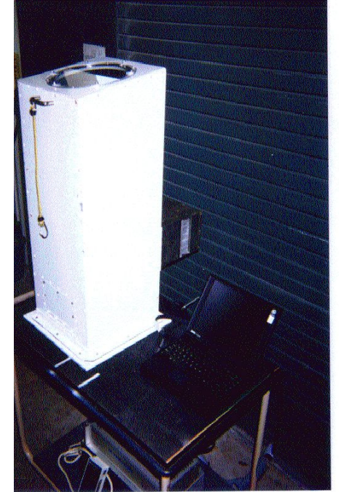
We built an environmental housing for the MPL, which was used throughout my grad school and post-doc.
