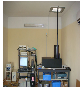
LIDAR Measurement of Depolarization and Backscattering Ratios.
