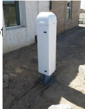
Ceilometer Measurement of Backscattering coefficient and Cloud base height .
