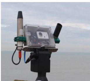
PANTHYR system [Vansteenkoven et al., 2019] 400-900nm, 10nm FWHM
