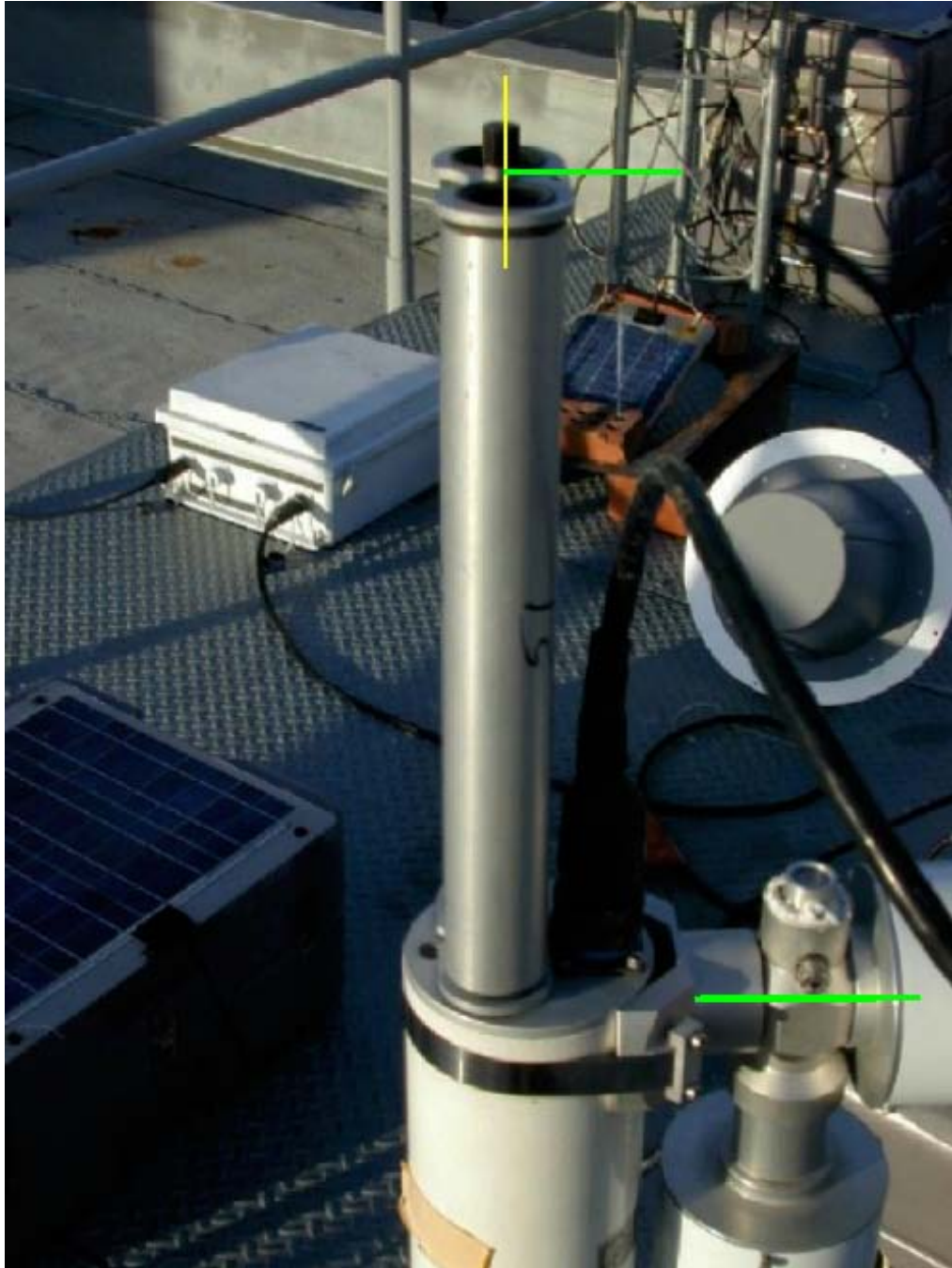
Figure 3 The long axis of the collimator cross-section (yellow) should be exactly perpendicular to the robot's zenith motor axis (green)
