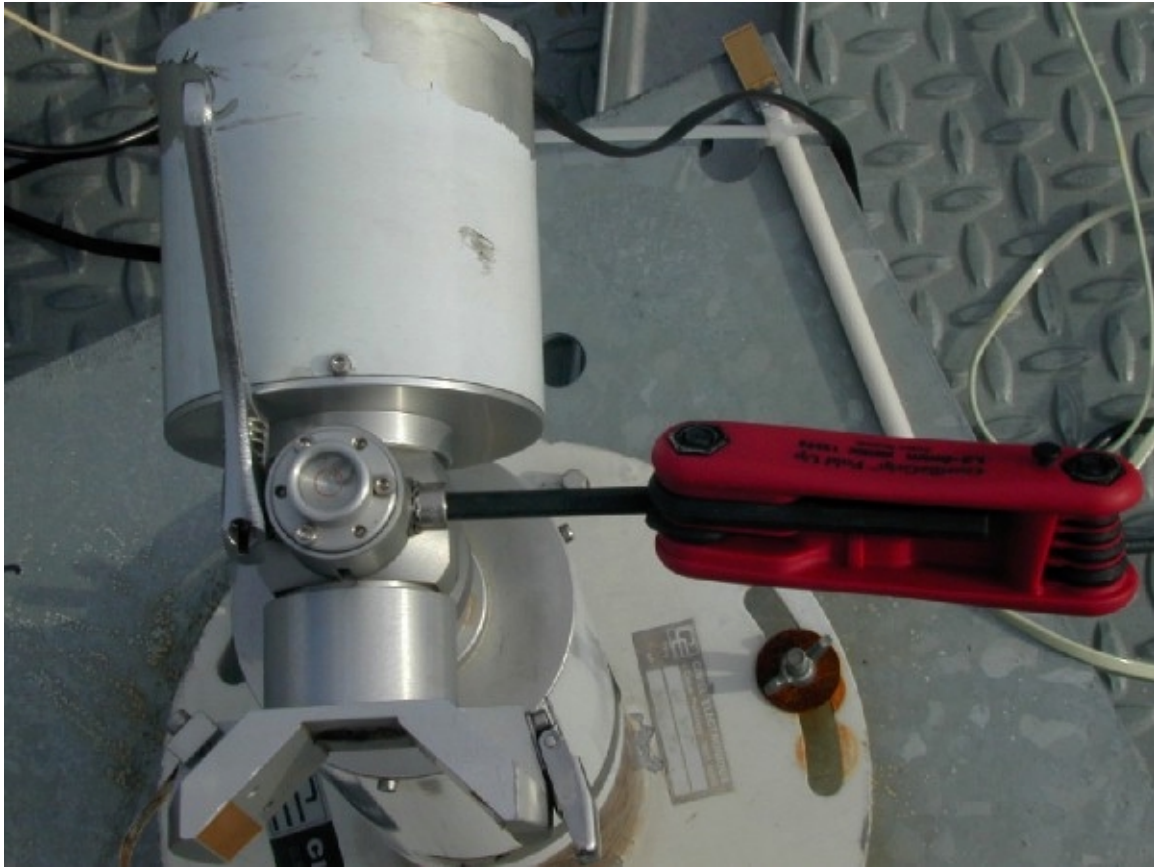
Figure 7: Adjusting zenith bolt
