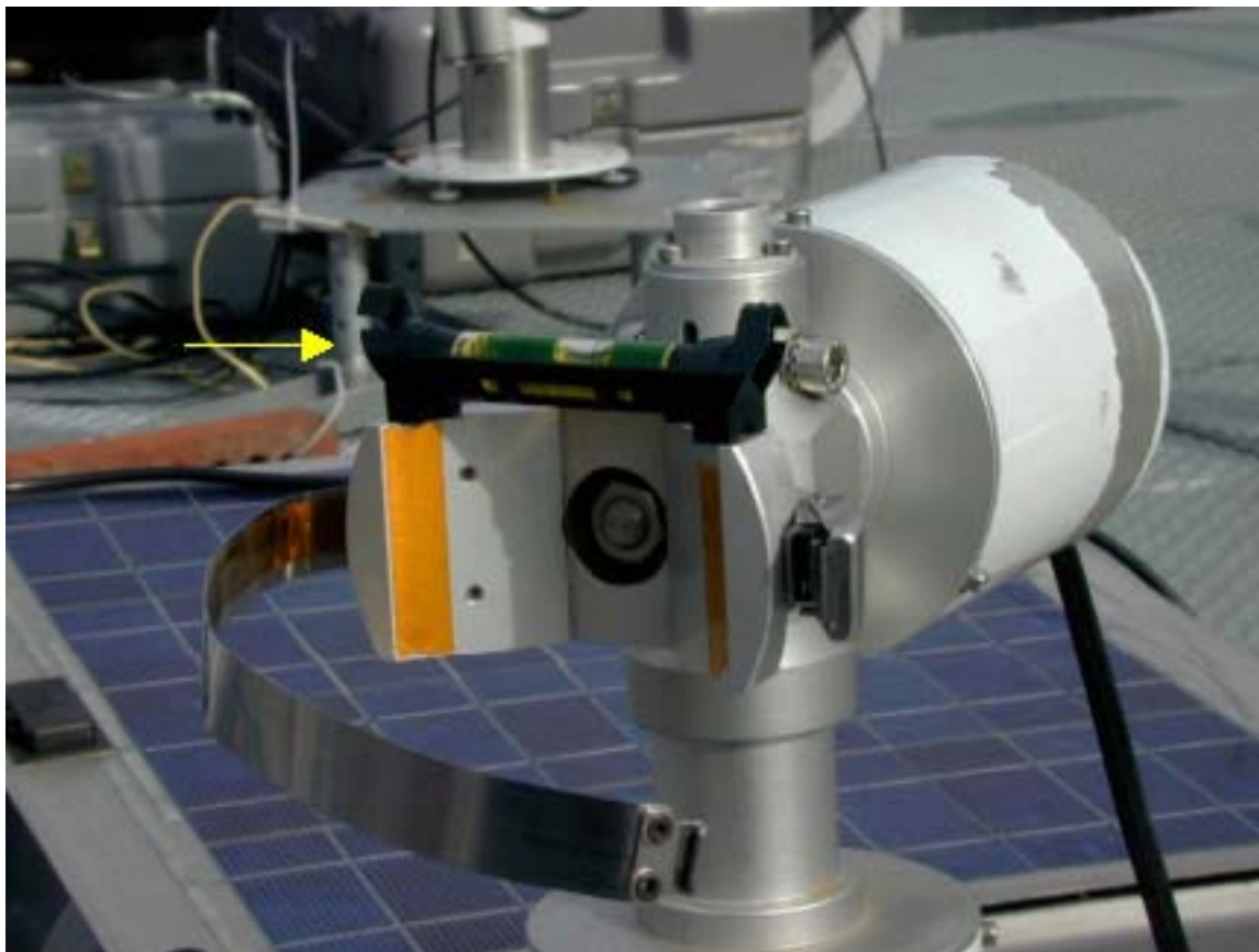
Figure 5: Leveling robot claw (sensor head attachment point)
