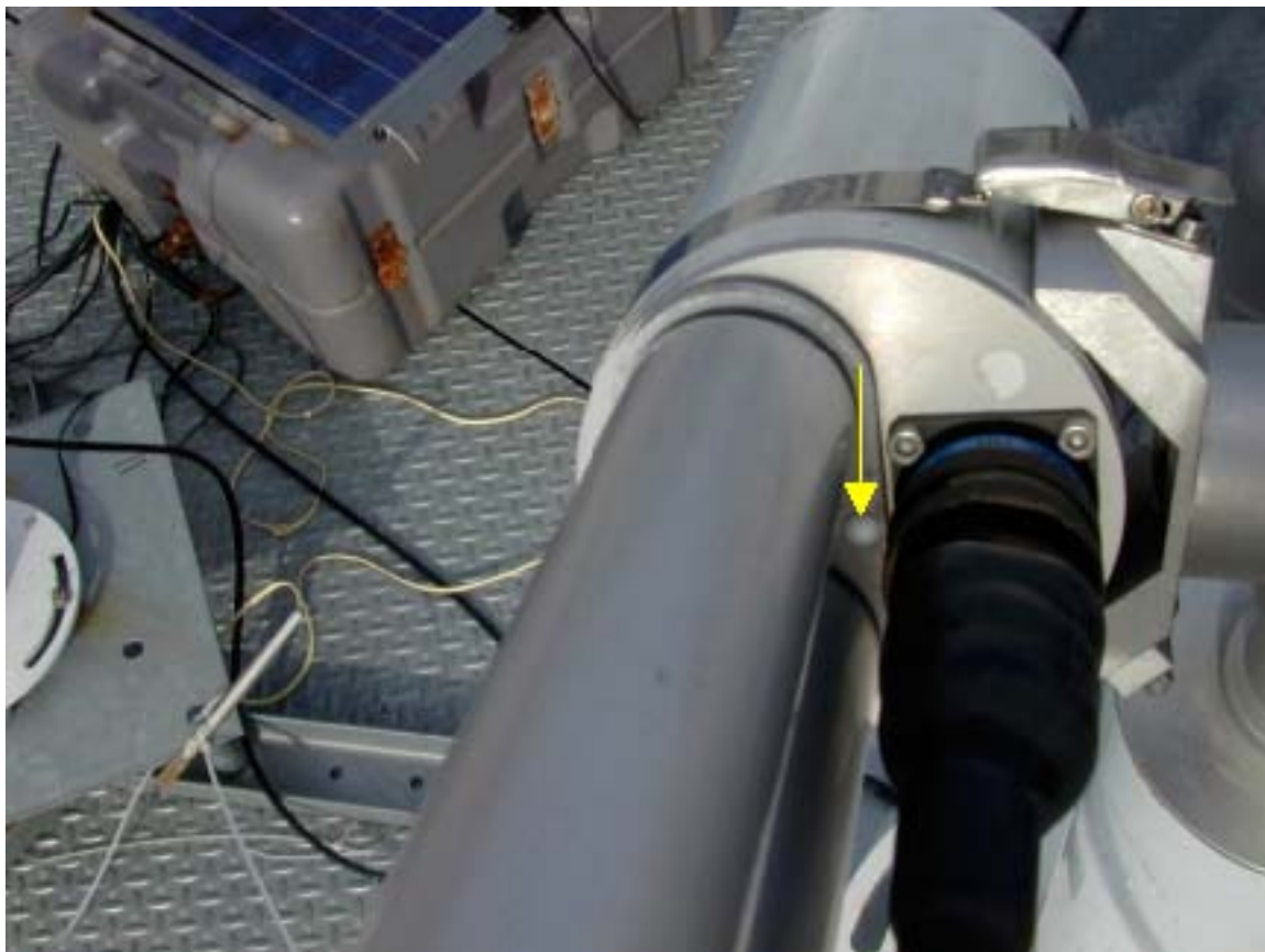
Figure 9: Sun spot from collimator centered on white alignment disk
