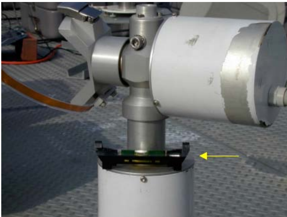
Figure 4: Leveling robot (Do not use top bubble level).
