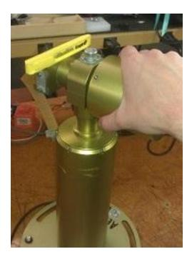
9. Once it is level, you should fully tighten the two underneath nuts of the newer robots, or nut 2 of the older robots, shown below:
