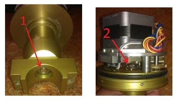
3. b) On the older model robot, you will need to remove the bubble level in order to access nut 1. Simply remove the three small screws holding it in place and it will come off. You may also need an extension to the socket wrench to reach nut 1, as shown below. Nut 2 can be accessed in the same manner on both models.
