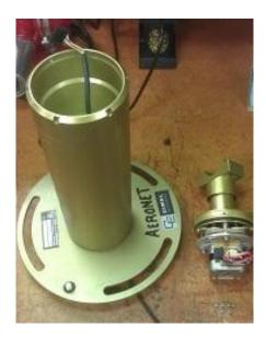
3. a) We now proceed to tightening the AZ drive. The bolt runs the length of the drive, and is secured on either end by the nuts shown below. Accessing nut 1 is the only difference between robot models. On newer models, accessing this nut is straight-forward, as shown below.
