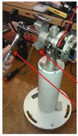
As you tighten nut 1, nut 2 will attempt to turn counterclockwise, but will be braced by the wrench and the post
