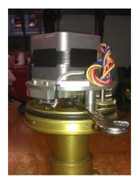
You should then be able to grip the clamp portion of the drive and tighten nut 1 with the socket wrench, with the 9mm wrench against the post holding nut 2 in place. This will cause both nuts to become tight as you tighten nut 1. Tightening as much as possible by hand should be sufficient. Remove the small wrench that you have holding nut 2, and you should now notice significantly more resistance if you try to rotate the drive.
