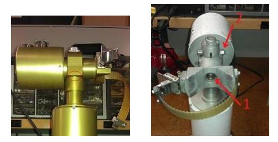
6. If you skipped here from the beginning of the guide, consult the pictures above and slightly loosen the circled nut (and the corresponding nut on the other side of the robot) OR the nut marked as 2, depending on your type of robot.
