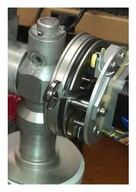
You should then be able to grip the clamp portion of the drive and tighten nut 1 with the socket wrench, with the 9mm wrench against the post holding nut 2 in place. This will cause both nuts to become tight as you tighten nut 1. Tightening as much as possible by hand should be sufficient. Remove the small wrench that you have holding nut 2, and you should now notice significantly more resistance if you try to rotate the drive.
