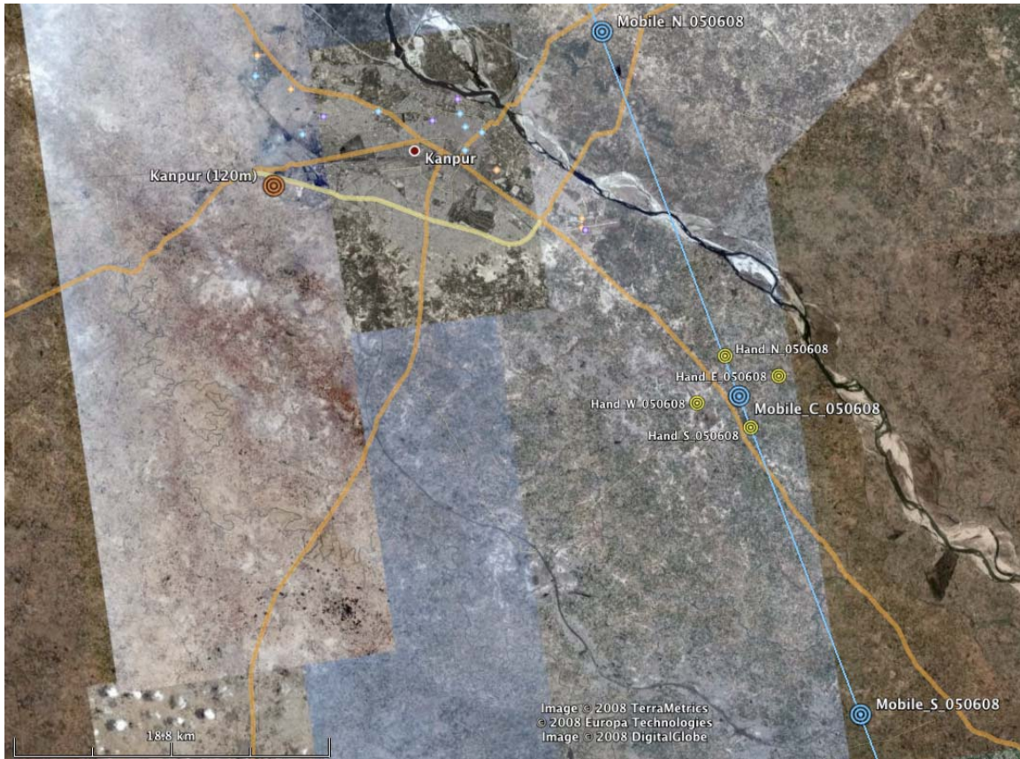
Figure 3 shows the three mobile sites (blue bulls eye) approximately 20 Km apart and the four handheld sunphotometer sites (yellow bulls eye) ~2.5 km around the central mobile site.
